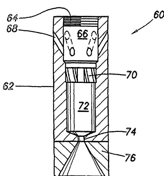
(57) Abstract: A jet nozzle is provided for drilling holes through the earth, such as drainholes around a well. The nozzle may include orifices for discharging fluid to drive the nozzle forward and includes a disk or other device having orifices to produce a swirling motion to fluid in the body of the nozzle. Swirling fluid is discharged from a front orifice and an extension is placed forward of the front orifice to confine the swirling fluid in a radial direction.
